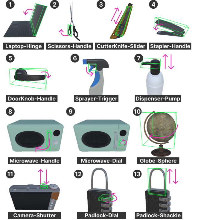
Figure 4: Selected 13 object-part pairs for user experience data collection in Study 1. Green bounding boxes show collider/trigger regions defined based on the mesh size of each part. Pink arrows indicate embedded motion constraints, which we predefined according to the natural behavior of each object (straight arrows for translation and curved arrows for rotation).
